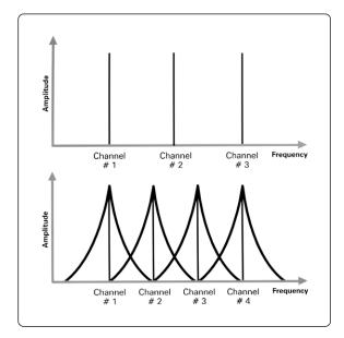
Figure 3. Smaller channel spacings mean greater need for spectral purity
