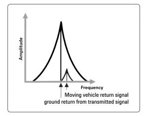
Figure 11. The effect of phase noise on radar
