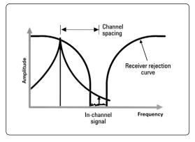
Figure 5. Out-of-channel phase noise causes in-channel distortion
