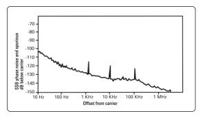
Figure 2. Signal generator SSB phase noise and spurious
