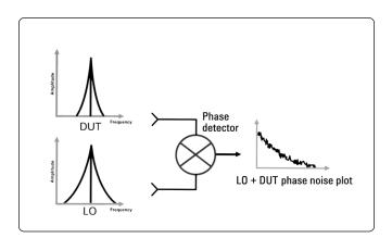
Figure 12. LO noise adds to the noise on the DUT
