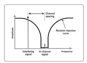
Figure 4. Receiver IF pass-band with in-channel signal present
