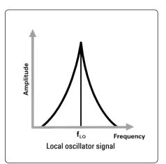
Figure 9. Local oscillator with phase noise
