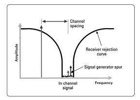
Figure 6. In-channel spurious signals makes a receiver look worse than it is
