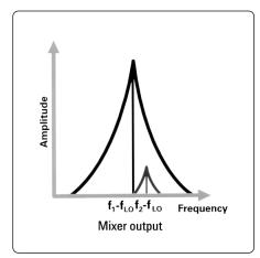
Figure 10. Phase noise masks the lower-amplitude signal
